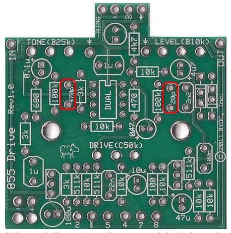
Step 5: Add the ceramic disc capacitors. These are not polarized and can be inserted into the PCB either way.
