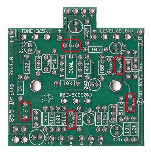
Step 5: Add the filmcapacitors. Film caps are not polarized and can be inserted into the pcb in either direction.
