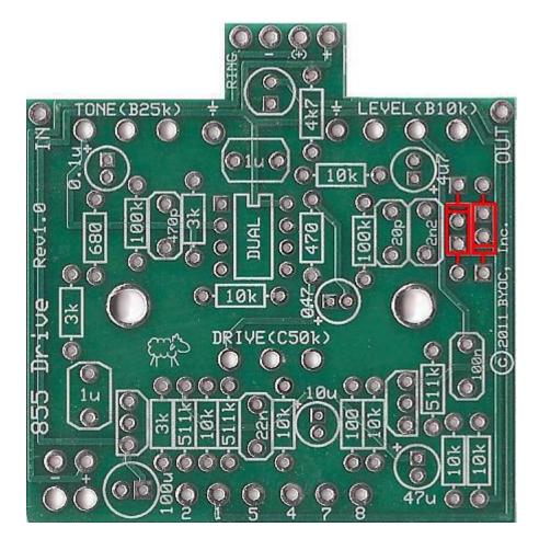
STEP 1: Add the 1N60 diodes. Be sure to matched the end of the diode with the stripe to the layout on the PCB. The stripped end should go in the square solder pad. Note that there are two additional through-hole solder pads within each space for the diodes. These are here for experimentation with other diode combinations. If you are building your 855 kit to stock specs, nothing will go in these additional solder pads. The 1N60 diodes should lay right on top of the additional solder pads.
