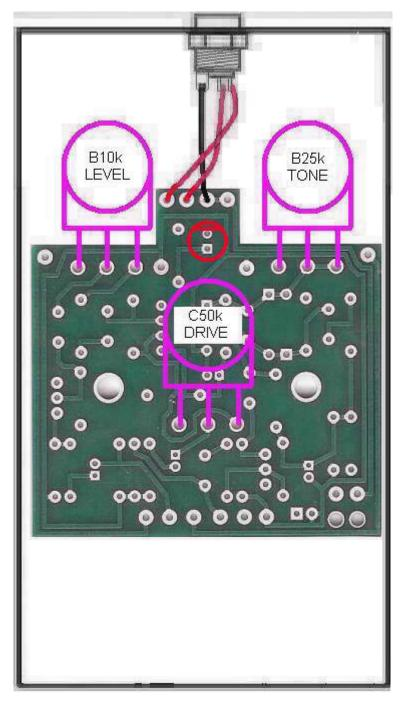
Step 3: Flip the PCB over so that the bottom or solder side is up. Insert the B100k(LEVEL),A500k(DRIVE), B25K(TONEI) potentiometers, and the LED into the bottom side of the PCB. DO NOT SOLDER ANYTHING YET!!! The LED will have one lead that is longer than the other. The longer lead goes in the hole with the square solder pad.
