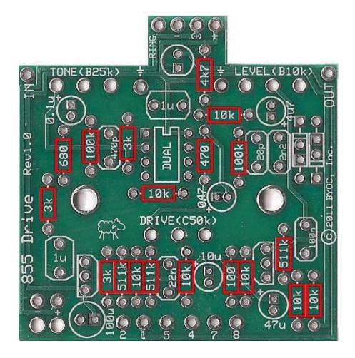
STEP 2: Add the resistors . Resistors are not polarized, so it does not matter which end goes in which solder pad. Take your time and be sure not to confuse similarly banded resistors such as the 100 ohm with the 100 k. This is a very common mistake.
