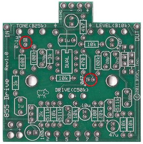
Step 6: Add the tantalum capacitors. Tantalum caps are polarized. The positive lead goes in the square solder pad hole. The positive side will have a stripe running down one side and the "+" symbol above the positive lead.
