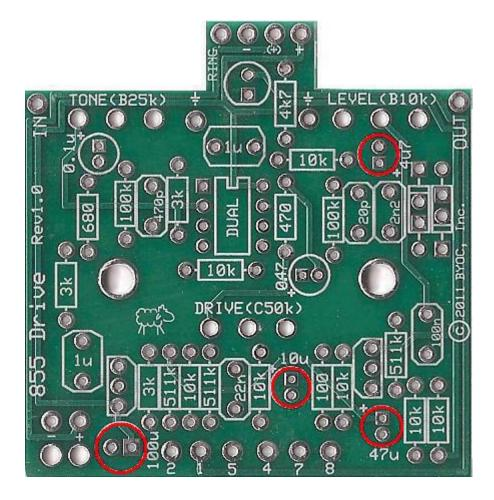
STEP 6: Add the aluminum electrolytic capacitors. These are polarized. The positive end will have a longer lead and should go in the square solder pad. The negative end will have a shorter lead with a black or white stripe running down the body of the capacitor.
