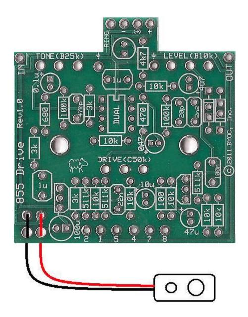
Step 7: Add the battery snap. Thread the solder ends of the battery snap into the strain relief holes from the bottom solderside of the PCB and out through the top. Insert the solder ends of the battery snap wires into the topside of their respective solder pads. Solder on the bottom side of the PCB. Remember the red wire goes in the "+" hole and the black wire goes in the "-" hole.
