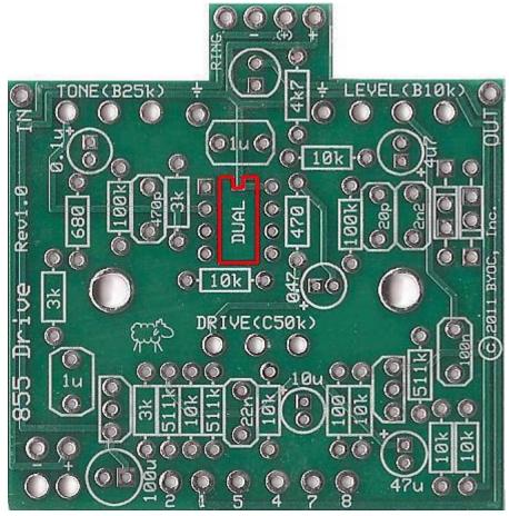
STEP 3: Add the 8 pin IC socket. **ONLY SOLDER THE SOCKET! NOT THE ACTUAL IC!** This is a socket. The sockets get soldered to the PCB. The ICs get inserted into the sockets. The actual IC chip itself, never gets soldered. You will insert the IC into the socket after the entire pedal has been built.
