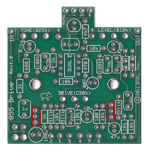
Step 4: Add the Transistors. Be sure to orient the transistors so that the flat side of the tansistor body matches up with the flat side on the PCB layout.
